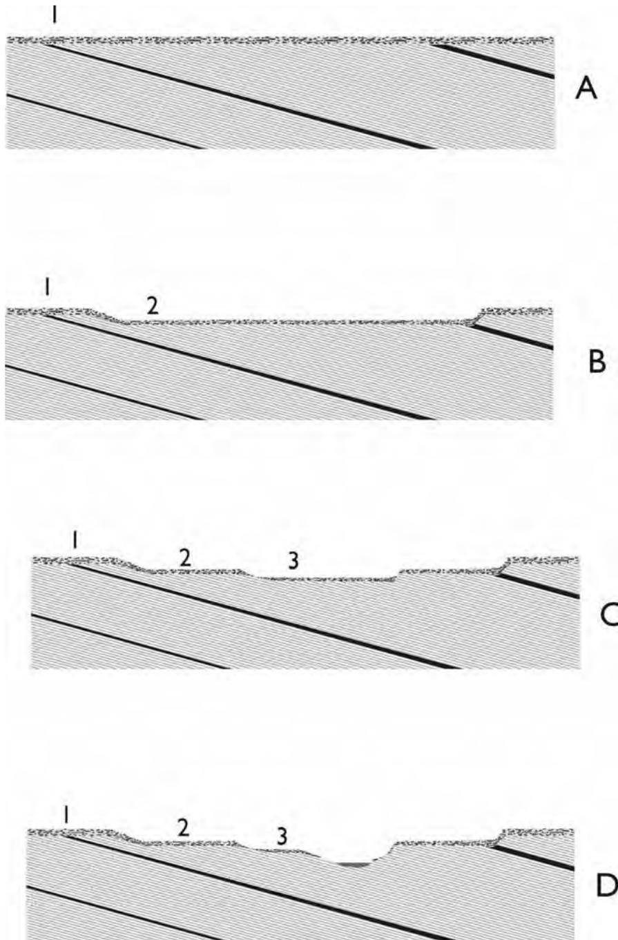
**Figure 3.** The formation of three strath terraces in a river valley. (A) The river first erodes a nearly flat planation surface, or “strath,” on hard rock and deposits a thin veneer of coarse gravel across the entire valley. (B) The river erodes some of the bedrock, leaving strath terraces on either side of the valley. (C) A second erosional event creates a second set of strath terraces. (D) A third episode forms a third set of strath terraces. (Drawn by Peter Klevberg)
