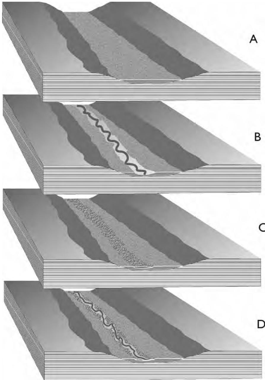
**Figure 1.** The formation of two gravel terraces in a river valley. (A) The river valley is first carpeted with a layer of coarse gravel. (B) The river erodes this gravel, leaving gravel terraces on either side of the valley. (C) A second depositional event partially fills the eroded valley with coarse gravel. (D) The river erodes the second layer resulting in new gravel terraces. (Drawn by Peter Klevberg)
