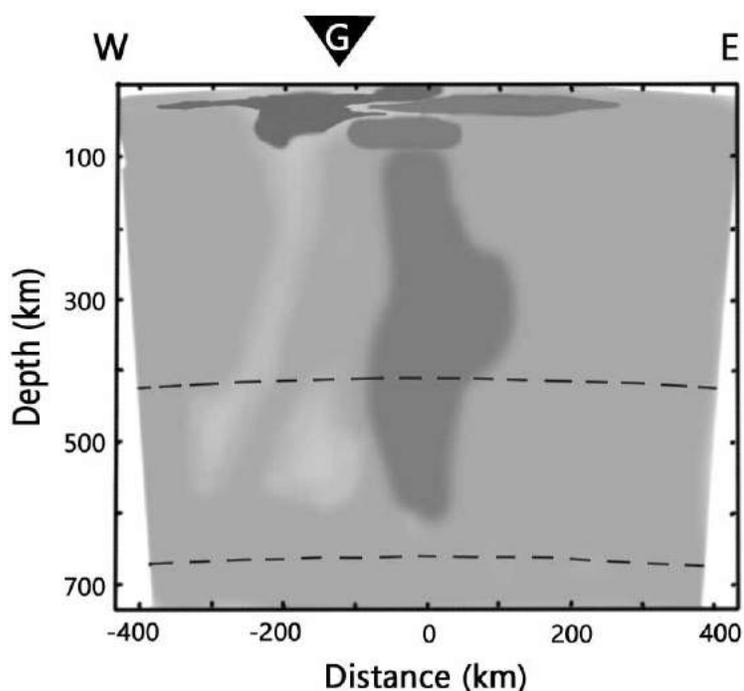
Figure 9. A west-east vertical tomographic image through the Alboran Basin showing the vertical slab of high seismic velocity that starts near 60 km deep and extends to about 650 km. (Copyright 2013 from Bezada et al., 2013, p. 55, and modified by Mrs. Melanie Richard. Used in accordance with federal copyright [fair use doctrine] law. Usage by CRSQ does not imply endorsement of copyright holder.) “G” is the location of the Strait of Gibraltar.
