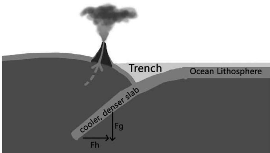
Figure 8 (left). Horizontal and vertical components of the slab pull force. It is  $F_h$  that is supposed to cause slab rollback (also called trench or subduction rollback.) Drawn by Mrs. Melanie Richard.
