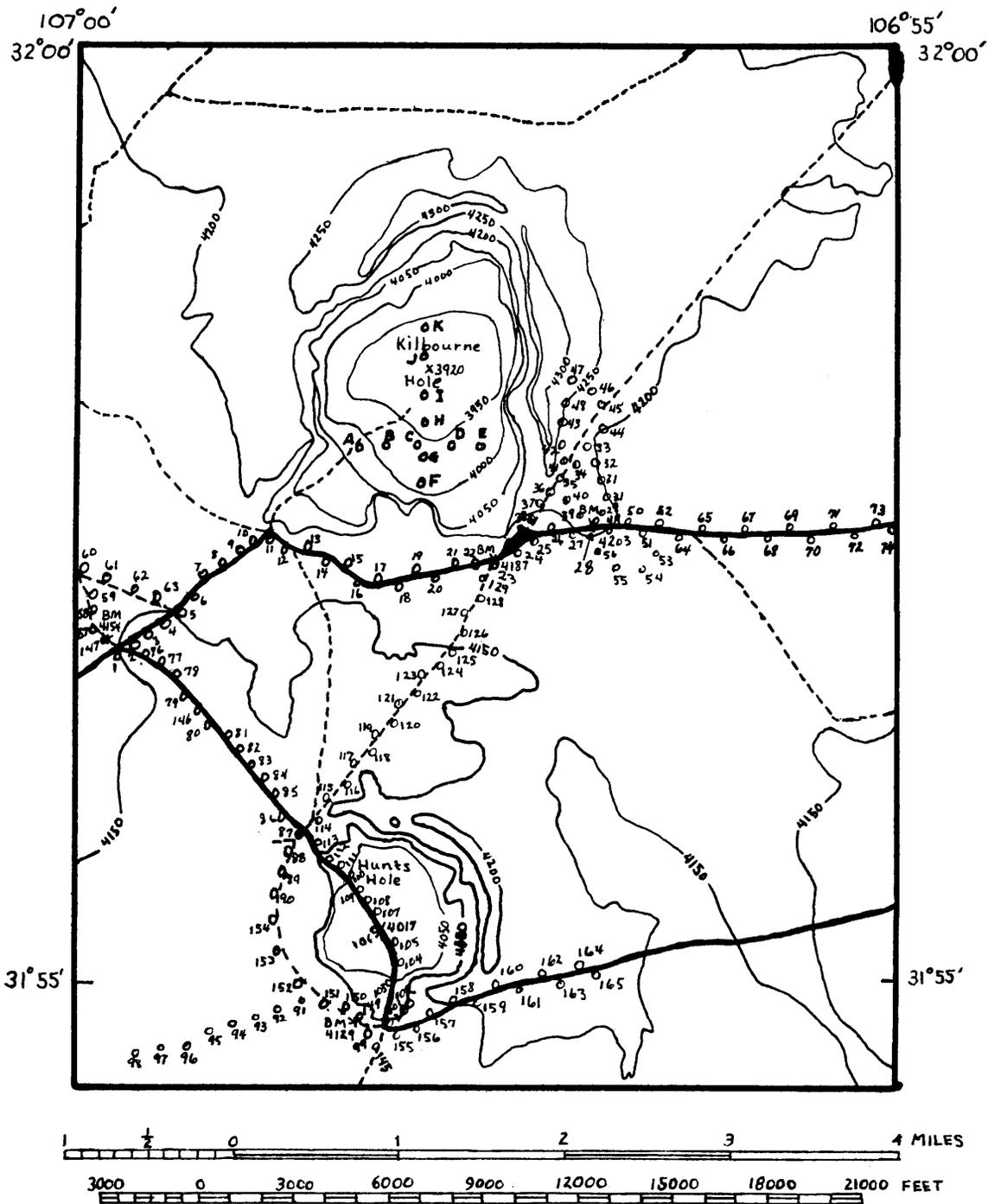
THE SMALL CIRCLES INDICATE THE LOCATION OF THE GRAVITY STATIONS. TABLE 1 GIVES THE GRAVITY VALUE IN MILLIGALS FOR EACH STATION RELATIVE TO STATION 28.
