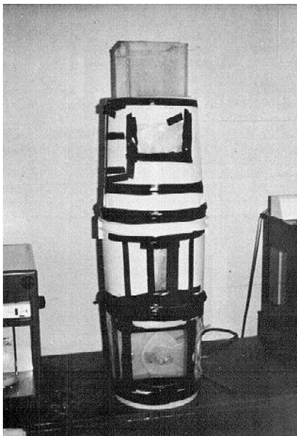
Figure 1. Apparatus used to ensure a wet environment around the precipitation area.
