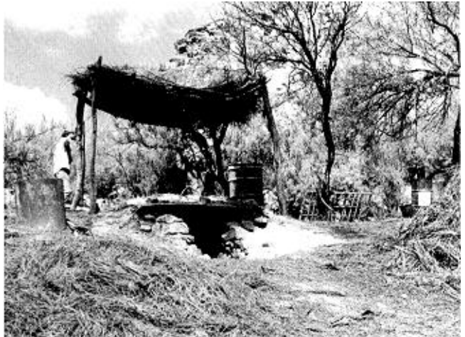
Figure 15. Candelilla wax extraction facility. A fire is produced in the pit seen here. Candelilla stems are placed in a boiling sulfuric acid solution above.
