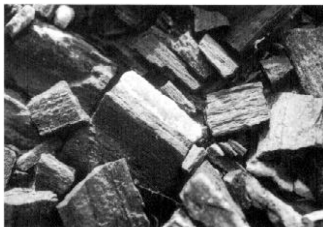
Figure 1. Pieces of silicified wood that have disintegrated from a recently exposed log in the Dawson Creek region of Big Bend National Park. Light areas are fairly pure (~97%) silica that probably filled cavities within the log. Photograph by Glen Wolfrom.
