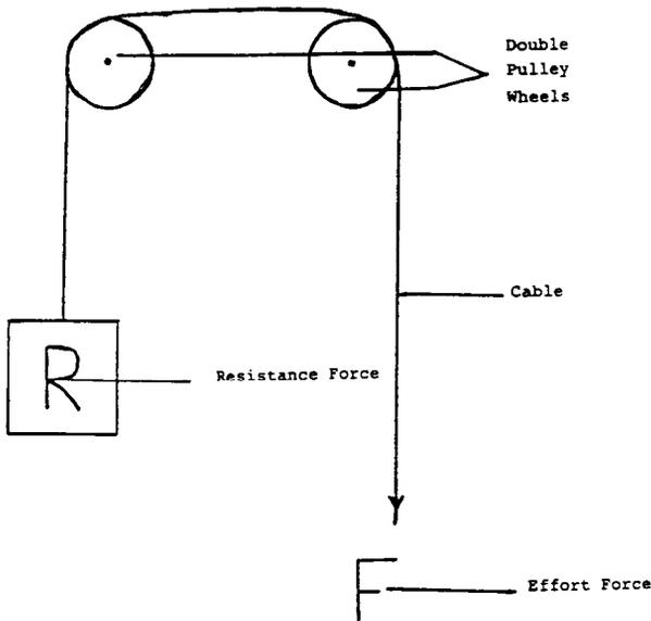
Figure 2. Double pulley.
