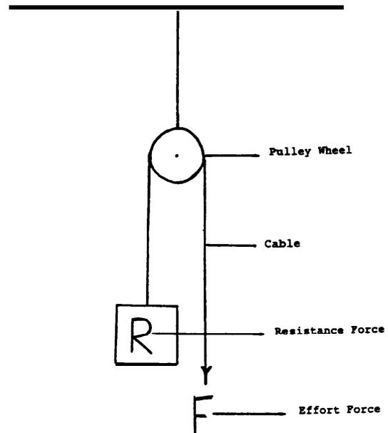
Figure 1. Simple pulley.
