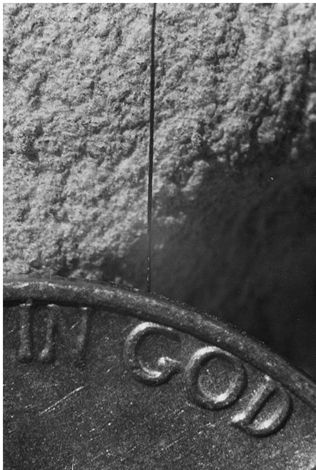
Figure 3. Photomicrograph of a dime and a human hair on the rim of the arch of track 39, for size calibration at about 15X. Hair is about 100 microns wide.
