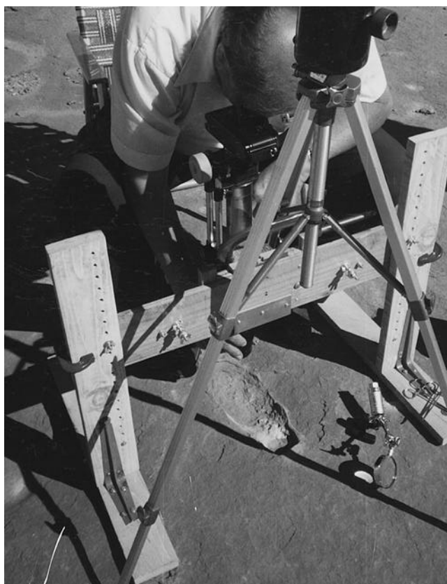
Figure 1. Davis prepares to photomicrograph track 39. The heavily weighted tripod steadies the camera apparatus. The spot being photographed was lit by the sun via a magnifying glass.
