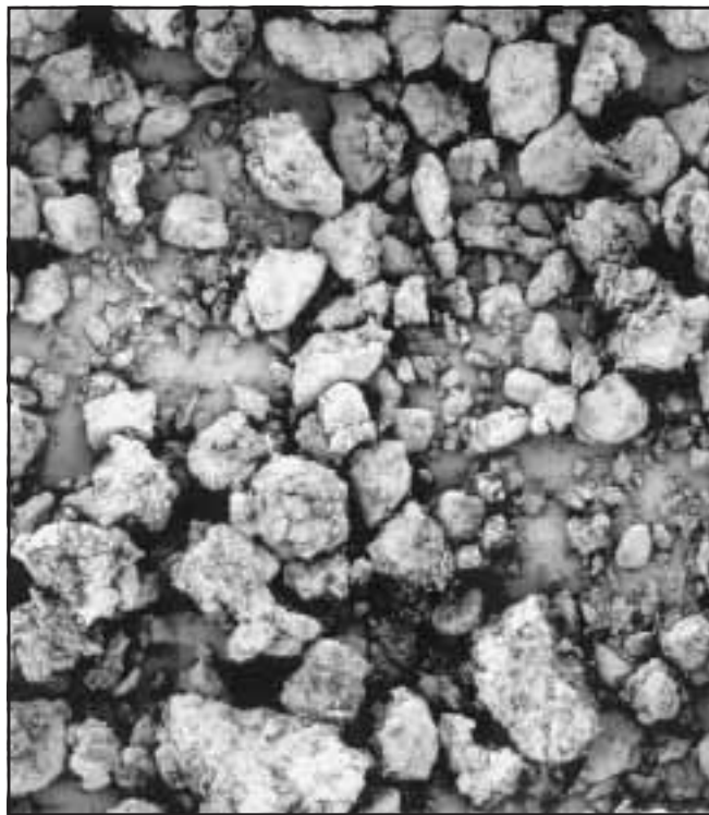
Figure 12 Scanning electron micrograph of unweathered sample from mound M2. The sharp-cornered particles are quartz shards. Micrograph by William Stark. Magnification 40X.
