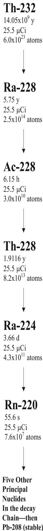
Figure 2. One mole of thorium (232.038 g) maintains under secular equilibrium 1 billionth of a microcurie of C-14 by the low-probability emission of C-14 nuclei from Ra-224. This is 9.8 million atoms of C-14 per mole of thorium that corresponds to a C-14/Th ratio of  $1.6 \times 10^{-17}$ . This diagram does not include the C-14 production by neutron activation of nitrogen.
