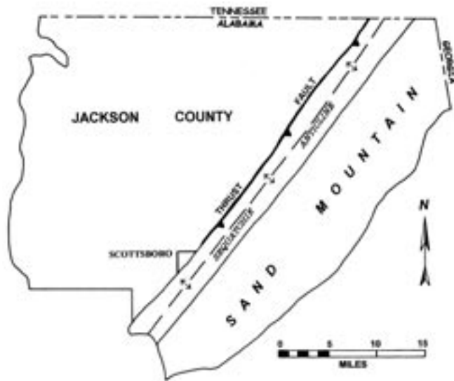
Figure 9. Trace of the Sequatchie thrust fault as it apparently ends north of Scottsboro, Alabama (after Thomas, 1972). Drawing by Mary Elizabeth Akridge.
