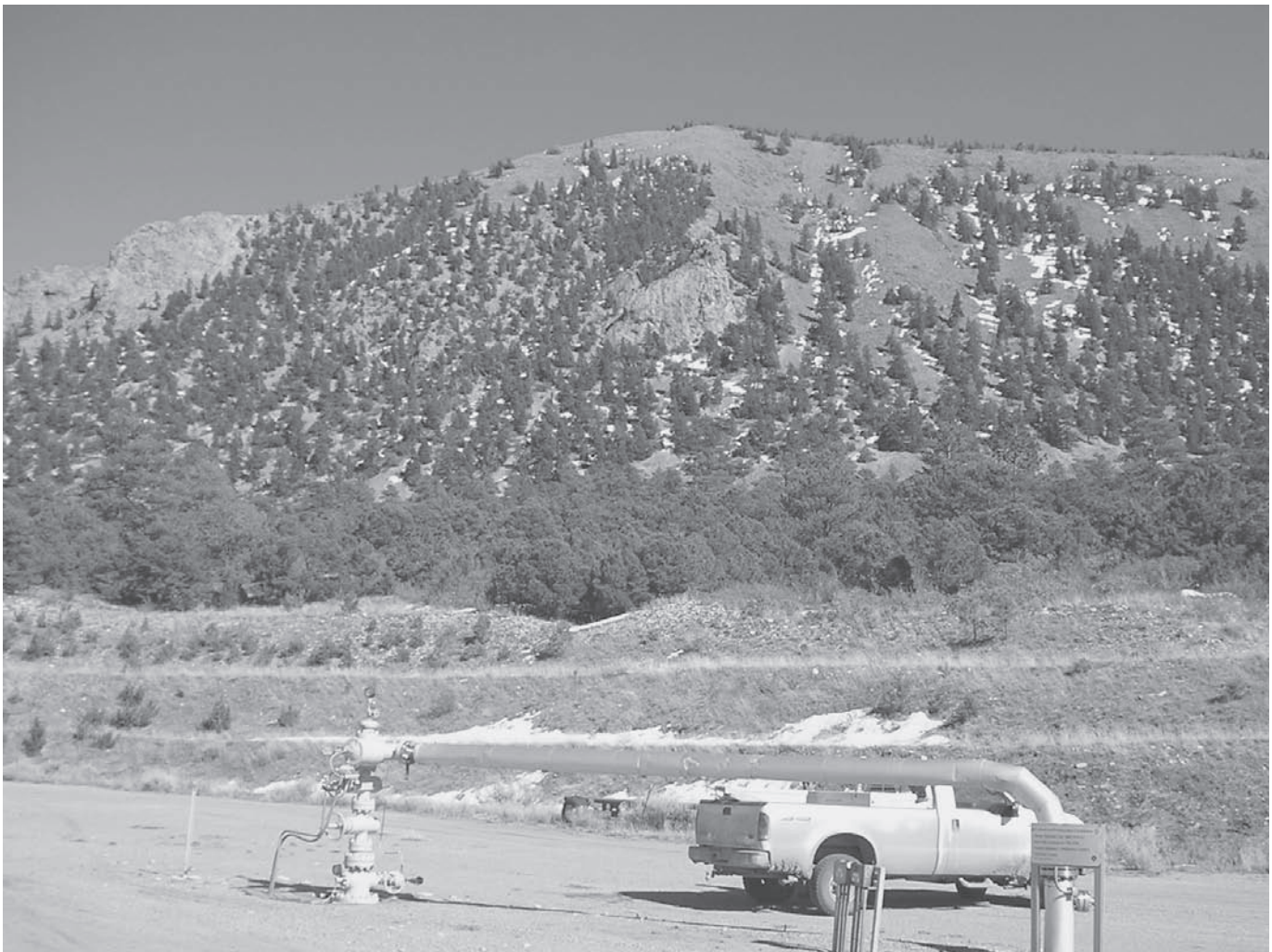
Figure 3. Sheep Mountain Field CO 2 gas well site. Little Sheep Mountain in the background. Many wells are slant drilled from one location.
