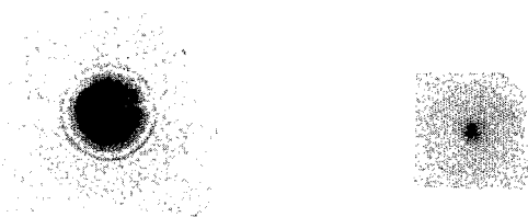
Figure 1. A uranium-238 halo (left) and a polonium-210 halo in biotite. Scale is 1 cm equivalent to 26.5 \mu m.
