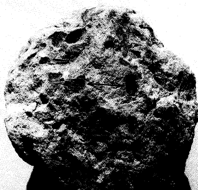
Figure 2. The dark hematite has served to preserve the wood grain orientation (shown by the arrow direction for the fragments to the left and right of the arrow). Some of the wood fragments found within this layer have sharp fractures perpendicular to the wood grain, indicating that they are likely to be derived from charcoaled wood and not green wood.
