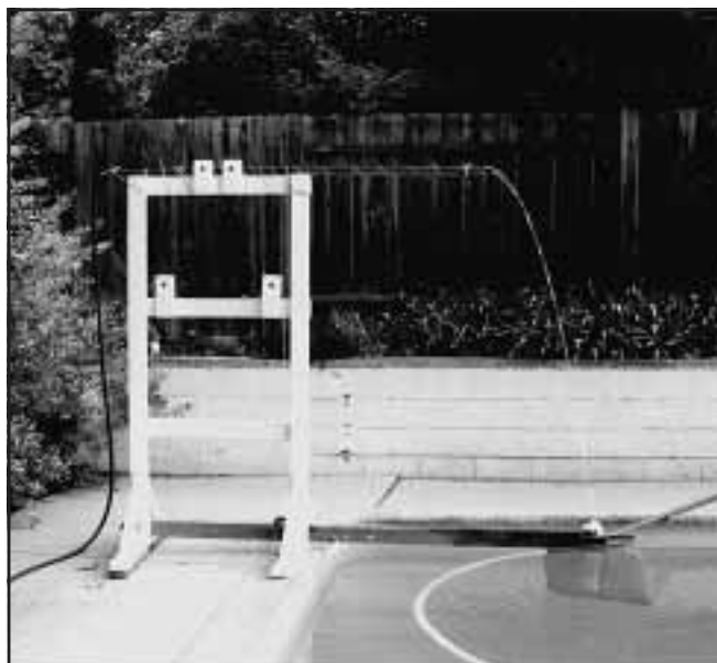
Figure 2. Experimental setup. The vertical and horizontal distances are 176 and 50 cm, respectively.
