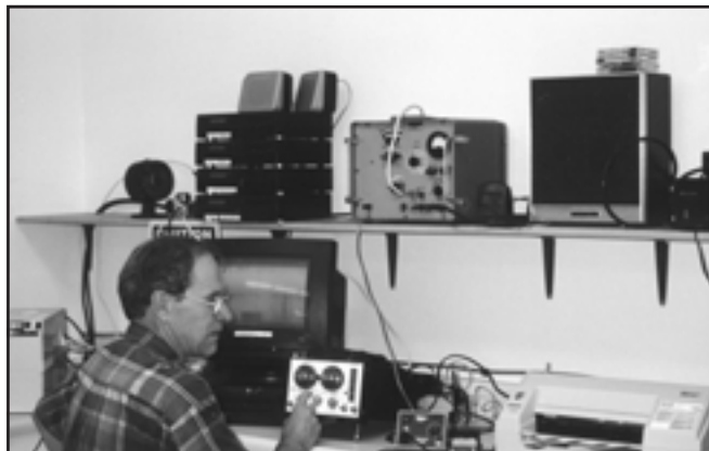
Figure 6. Jack Meyer, visiting scientist from Virginia, puts finishing touches on the Stardust Radiometer observation station. Stardust detects and automatically records about 3,000 incoming, high altitude, ionized meteor trails on an average day.
