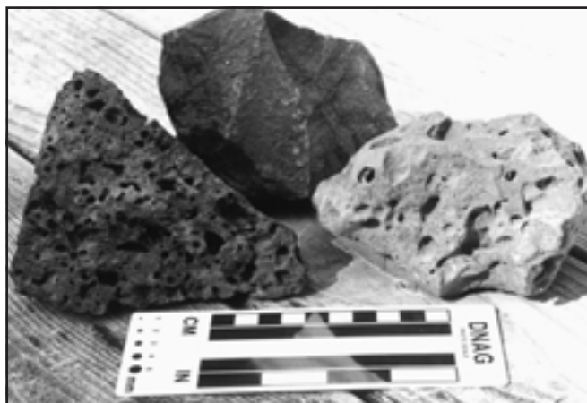
Figure 10. Basalt blocks with varying degrees of vesicles. The upper scale is in centimeters and the lower scale is in inches. These gas bubbles reflect the amount of volatiles present within the melt at the time the lava cooled.
