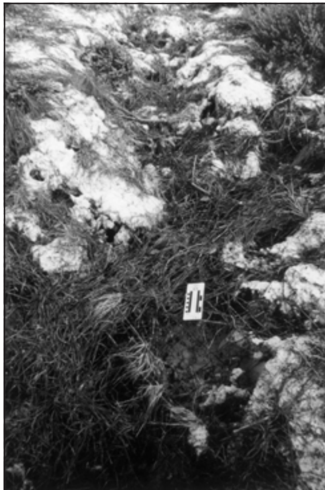
Figure 11. The scale is suspended eight to ten inches above the drainage channel, by a mat formed of pine needles lying on top of undamaged plant roots. After it fluidized, the sand was removed by dropping into the deepening channel, and then moving along the channel to the point of discharge.
