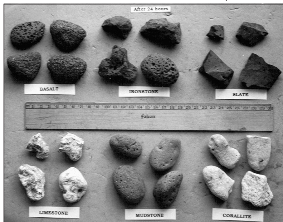
Figure 1. Rock samples after 24 hours of exposure to flowing water.
