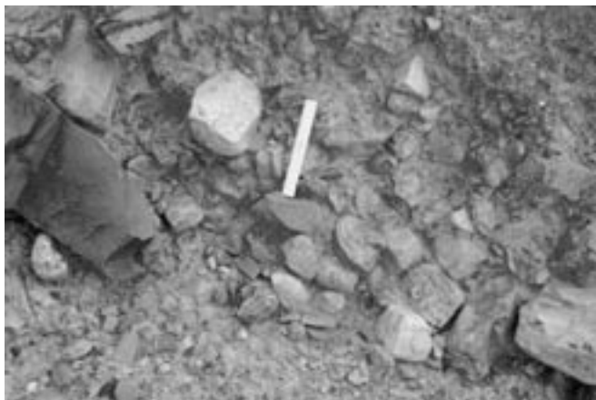
Figure 21. Angularity of Kennedy gravel—picture from Two Medicine Ridge. Scale is 16 cm (6 in) long.
