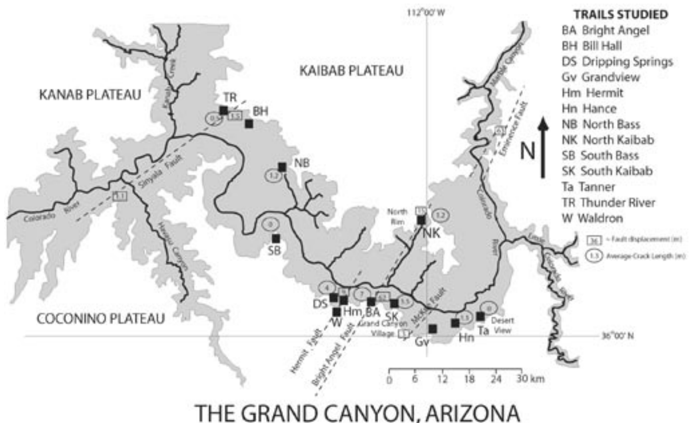
Figure 1. Trail locations and northeast trending faults, pertinent to this study. Sand-filled crack lengths are indicated by ovals and vertical fault displacements are indicated by rectangles. Fault locations are approximate.
