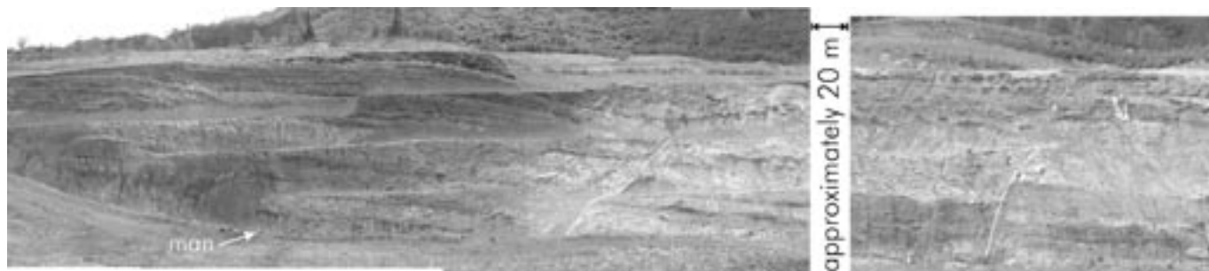
Figure 13. Panorama of the third coal mine starting from east and moving westward. Man for scale standing at the bottom of the excavated cliff at lower left. Note that the strata are evenly bedded with a minor fault toward the right. The section is about 30 m high and 500 m long.
