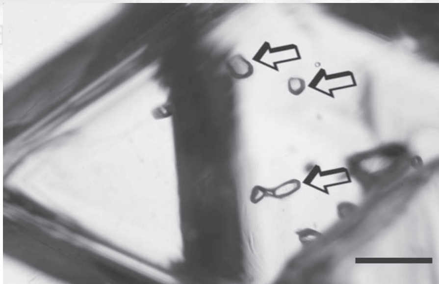
Figure 1. Diamond fragment with inclusions (possibly zircons – white arrows), from Orapa mine (world’s largest diamond mine in Botswana, Africa). Magnification 300X; scale bar = 200 micrometers.
