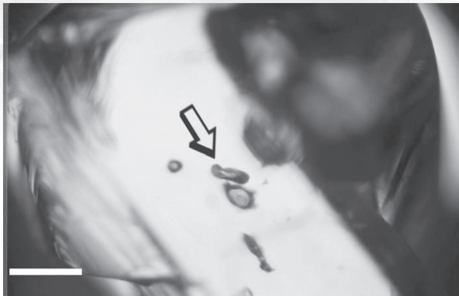
Figure 3. Diamond fragment with inclusions (garnets), from Orapa mine. Magnification 300X; scale bar = 200 micrometers.
