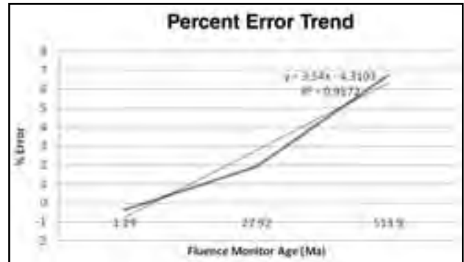
Graph 1. Percent error between the Ar and Age Ratios for various fluence monitors
