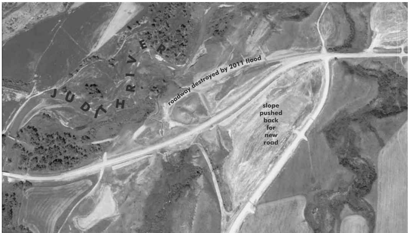
Figure 3. Aerial view of Hanover Road west of Lewistown, Montana, showing large amount of earthwork necessary to relocate road away from edge of valley where 2011 flood seriously damaged the road. Photograph taken 2014, obtained from Google Earth.
