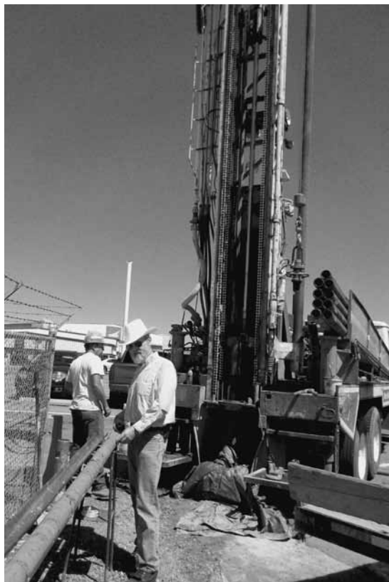
Figure 3. Lead author logging core from boring in basal (Flood Member) Blackleaf Formation sandstone. Sample G was obtained from slightly more than 9 m (30 ft.) into the sandstone bedrock.
