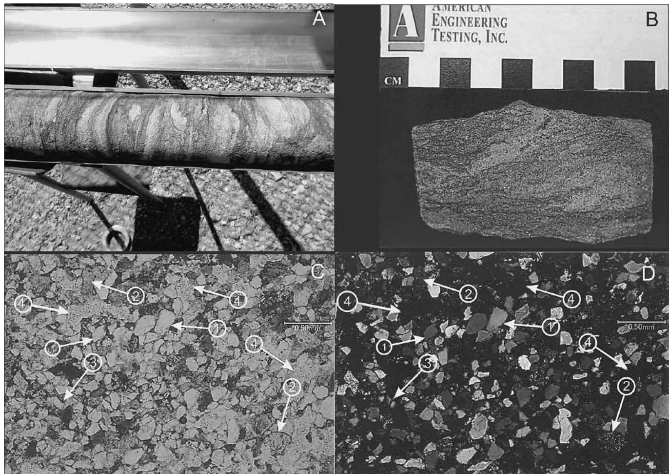
Figure 11. Sample G was collected from drill core obtained at the location shown in Figure 2 (47°29'05.85" North, 111°21'08.16" West). A is HQ core in tray. B is the section of core from which the sample was obtained, cut and lapped. C is thin section in plane polarized light. Arrows: 1 = detrital quartz, 2 = polycrystalline lithic fragments, 3 = feldspar, 4 = pore space. D is thin section in cross polarized light. The sample is a litharenite.
