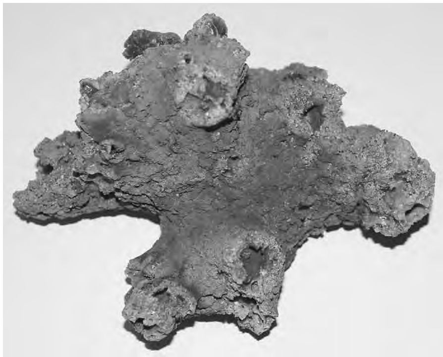
Figure 3. A fulgurite results from lightning striking the ground and fusing the sandy soil. This glassy sample is six inches (15cm) across
