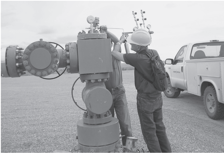
Figure 2. McElmo field, well# DC-9. One can see the two small 10 cc sample cylinders atop the sampling apparatus. May 29, 2014.
