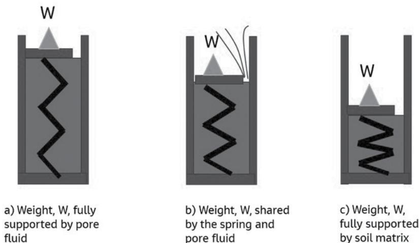
**Figure 1.** Three stages of consolidation: a) Initial loading where the load is transferred directly to the fluid (no load in the soil spring); b) load transfers from the fluid to the soil spring as water escapes; c) End of consolidation when all the load is now carried by the spring and no flow of water out of the soil
