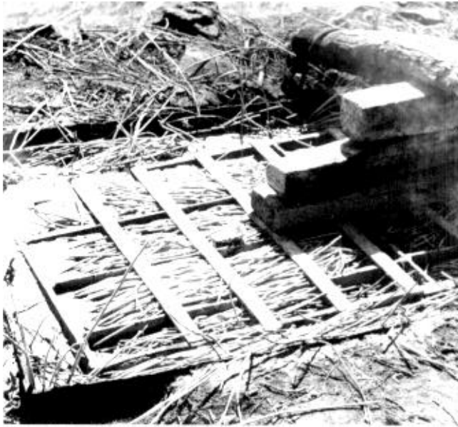
Figure 17. A grate is pressed by a lever to immerse candelilla stems into the boiling acid solution.
