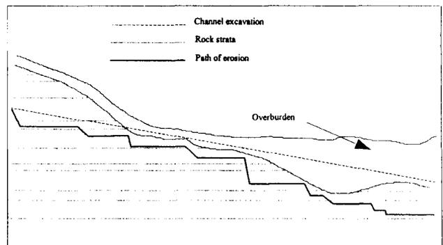
Figure 10. Hypothetical representation of erosion which may occur in a spillway outlet channel.
