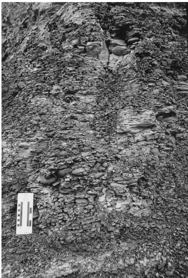
Figure 7. Closeup of the massive clays of the Pen Fm. Both vertical and horizontal joints were noted. Scale is in inches (right) and centimeters (left).
