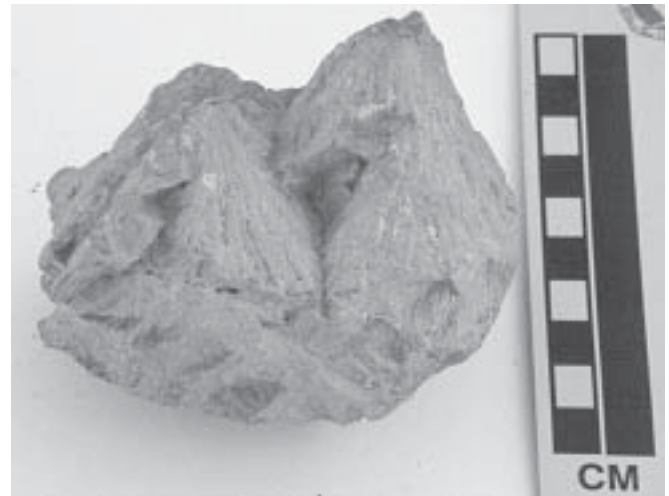
Figure 11. A photograph of two shatter cones in limestone collected from the Odessa Meteor Craters on display at the Gallery of Creation, Stone Mountain, Georgia. Scale in inches and centimeters. These features are indicative of impact craters and do not require exceptional impact forces to form them (French, 1998). The impact force propagates in an expanding manner and results in the formation of a cone-shaped feature. Scale in centimeters.
